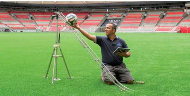
Figures 4 and 5: ball-roll and straight-edge test by a FIFA-accredited test institute prior to the FIFA Women's World Cup Canada 2015™
